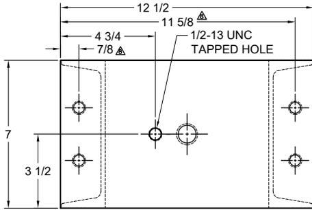
**TYPE MH-4C SPRING ISOLATORS WITH INTERNAL ADJUSTMENT**
